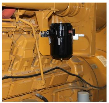
Naturally aspirated Fairbanks Morse OP engines have a selfcontained CCV system that meet the requirements of the EPA rule without modification
